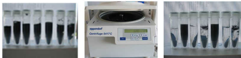
Fig. 1. Seven MWCNT-dispersions in water (left); centrifuge (middle); dispersions without or with suitable IL after 20000 rcf, 1 min (right).
