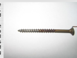
An Iron-screw, coated with Aluminium. © IOLITEC, 2005.
